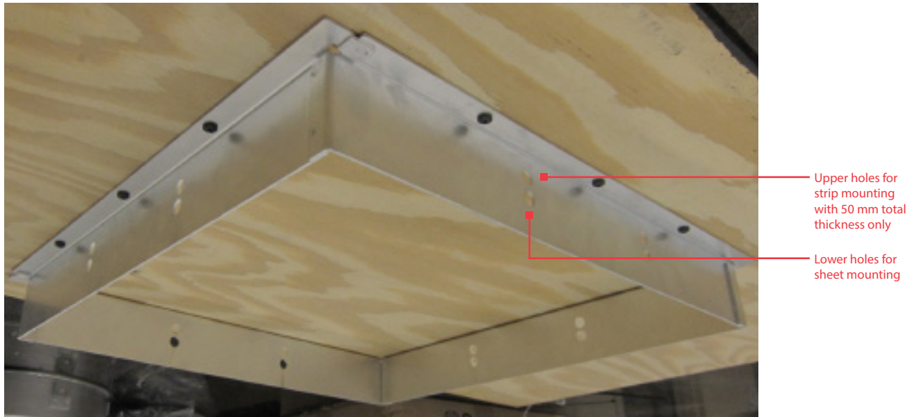
Figure 5: Incogneeto™ Frame Mounted Onto Plywood Sheet
